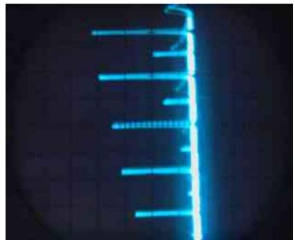
The photograph (right) shows the spectrum of the internal 10MHz crystal calibrator oscillator
