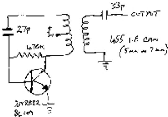
JFET circuit by Jim [G4MMH](#) 455kHz IF can to make a simple but effective BFO to resolve CW and S
