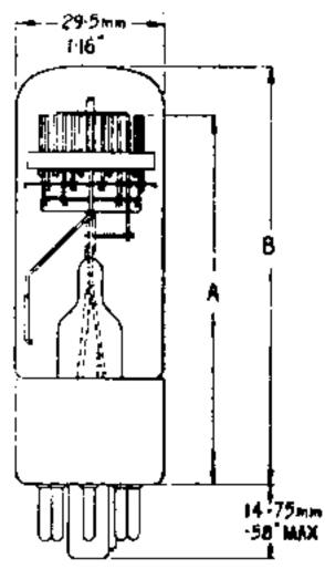
Dekatrons were used during the valve era for dividing by 10. The GC10B dekatron I have is capable of running at up to 4KHz. They work using a neon discharge between a pair of 30 electrodes. Every third electrode is connected such that using these three control signals it is somehow possible to move the glow around the circle. Other people have explained it far better than I ever could (or could be bothered to). Here's some references for further info:
